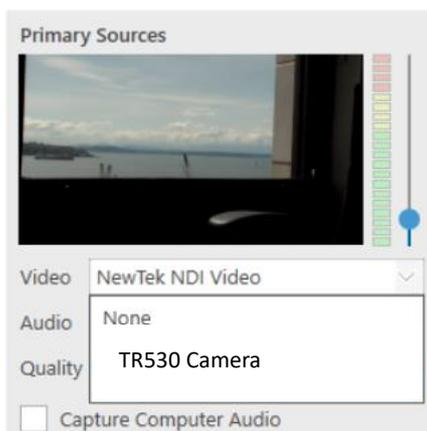
4. Next, you should be seeing the USB video from the TR camera. If you don't see any video, open *Device Manger* in Windows and verify the TR530 is listed under cameras.
