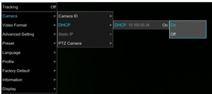
After turning DHCP on, go to **Information** to view the IP address.
