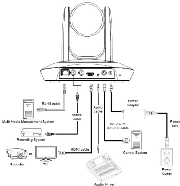
1. Connect the TR530 camera via RJ45 Network Cat5E (or better) cable; verify IP address of Camera in order to connect via Web browser. If IP address is not known, locate the remote, select the “Menu” icon and navigate to the “**Camera->DHCP->**” setting, verify DHCP is set to “On” in order to grab an available IP address. If you are reserving IP addresses, verify it is set to “OFF” and that the correct IP address has been set.
